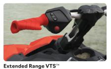
(Variable Trim System) Offers double the range of the regular  $VTS^{\text{\tiny{TM}}}$
